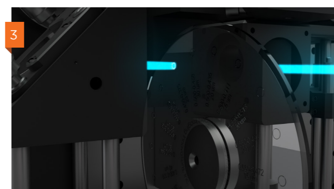
3 The annular mask acts as a zero-order filter, removing artifacts and lengthening the sheet.
