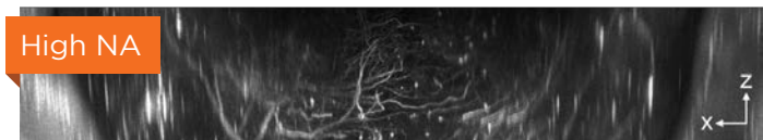
Thin static light sheet showing high resolution in the center of the field of view.
